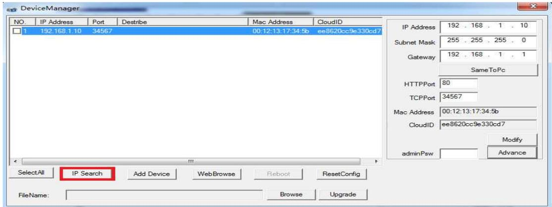
Step2: Modify IP address (make sure the IP camera and the computer in the same Network segment in one LAN)
